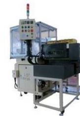
Tube Marking Machine 管刻印機
