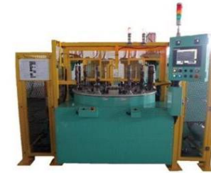
Auto Bottom Tube Brushing, Spraying, Drying, Leak Testing M/C 自動刷洗, 噴淋, 烘乾, 測漏機
