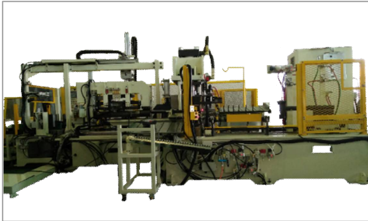
3-roll rolling/sizing/plasma welding Machine 3輪捲圓/整圓/等離子焊接機
