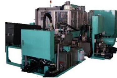
Auto Cylinder Feeding, Outer/Inner Brushing, Drying, and Tray Loading M/C 自動送料, 內外清洗, 烘乾, 工裝盤排列機
