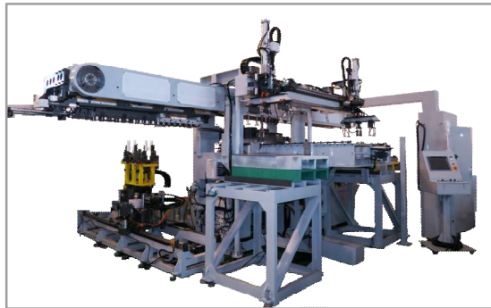
Double layer rolling/10 spot welding/flanging machine 雙層捲圓/10點焊/翻邊機
