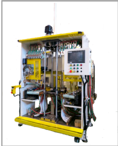
Press fit/8 spot welding for plate /2 spot welding for outer plate 插入/8點焊/2點焊
