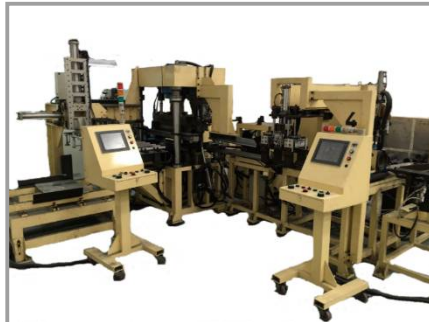
UO forming/plasma welding machine UO成型/等離子焊接機
